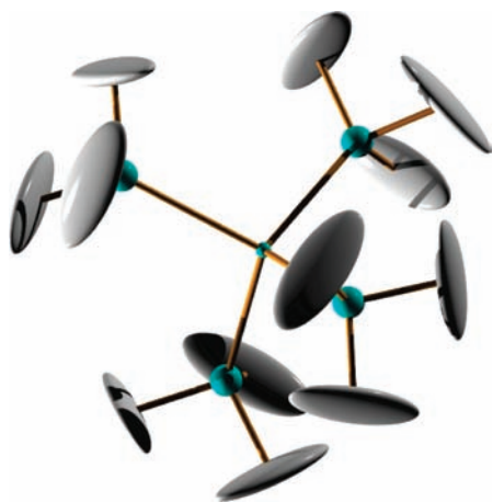
Figure 1. \text{Ga}(\text{GaH}_3)_4^{5-} cluster ion with a neopentane structure. At room temperature, very elongated thermal ellipsoids for the deuterium atoms indicate a significant librational motion of the \text{GaH}_3 units around the Ga–Ga bond. The view down the Ga–Ga bond shows that the \text{GaH}_3 unit is rotated \sim 11^\circ from the Ga–Ga angle in the cluster.
